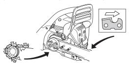
Make sure that the edges of the cutting links are facing forward on the top edge of the bar.
